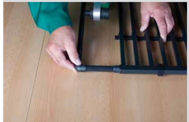
Fusion of pipe pieces
