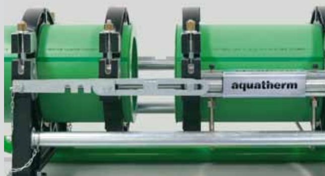
Divide the machine slide, remove heating element
