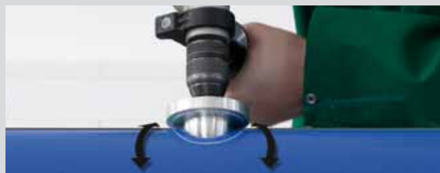
Removal of the oxygen barrier layer from the aquatherm blue pipe or
