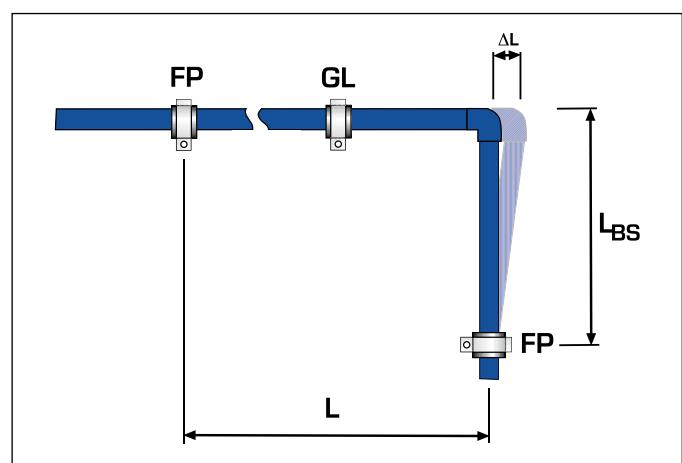
Calculational determination of the bending side length
