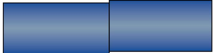
The misalignment cannot be more than 10 % of the wall thickness or max. 2 mm
