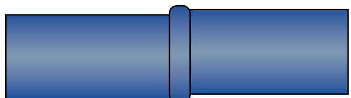
Misalignment of the joining area
