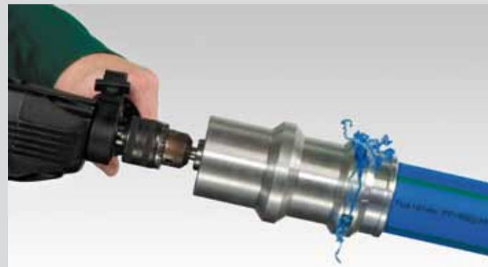
aquatherm peeling tool (Art.-No. 50558-70, up to 75 mm) (from 90-160 mm: Art.-No. 50572-50592 (without picture))
