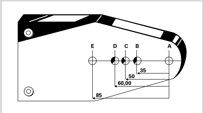
5. Place the welding tools on the welding device so that there is full surface contact between the welding tool and the heating plate. Welding tools over Ø 40 mm must always be fitted to the rear position of the heating plate.
