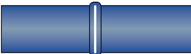
Lack of fusion at the joining area
