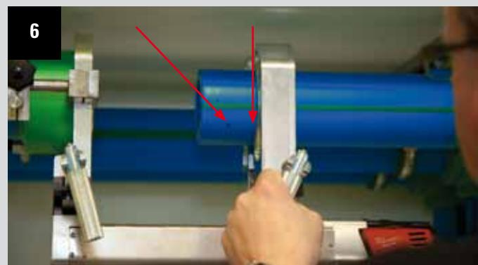
Lock pipe and fitting by using the front adjusting screws. (Fig. 7)
