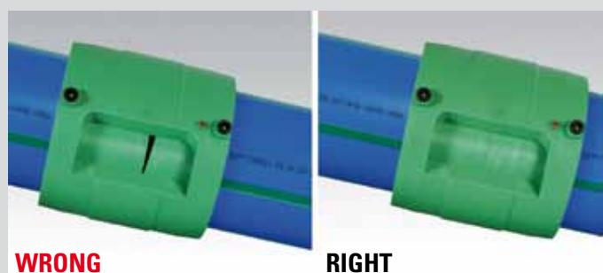
For a stable welding result it is important that both pipe ends inside the electrofusion socket are with parallel faces! Follow the minimum welding depth - absolutely!
