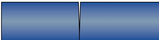
Gap width up to 355 mm outer diameter = 0.5 mm
